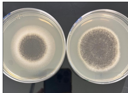
ASPERGILLUS BRASILIENSIS AT LEFT : STANDARD POTATO DEXTROSE AGAR AT RIGHT, WITH HEMP PEPTONE
