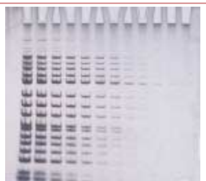
Sample: Marker 9 ( \phi X174/ Hinf I) digest 500, 250, 125, 63, 32, 16, 8, 4, 2, 1, 0.5, 0.25 ng/lane, respectively, from the left 6% of polyacrylamide gel (140×140×1mm) TBE buffer
